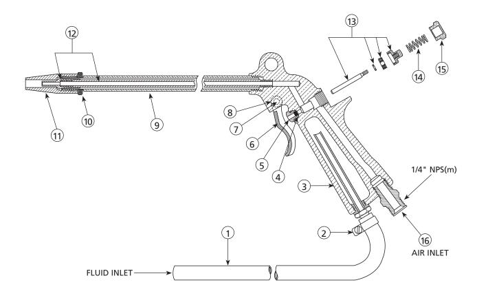
The Binks Model 140B spray gun is used for spraying solvents to clean engines and other machinery. Gun has a brass body with a ten inch nozzle/tube length. Flexible tubing is attached to the gun handle with a hose clamp for
