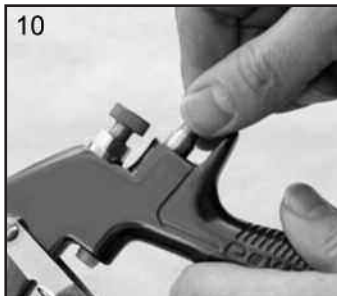
10. Fit new Seal to gunbody and press firmly to ensure Seal is engaged.
