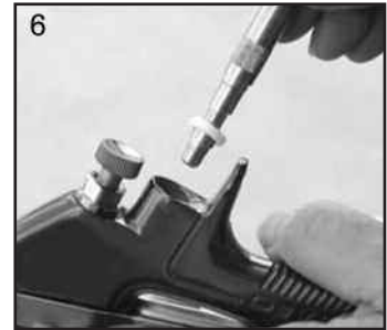
6. Remove Valve Seat.
