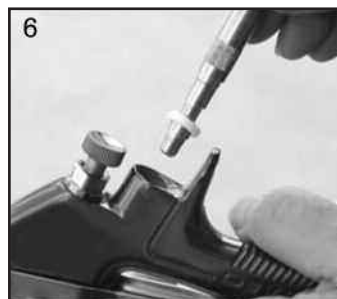
6. Retirer le support de la soupape.
