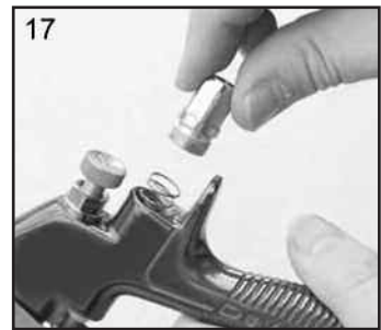
17. Replace Valve Spring and screw in Housing (10).
