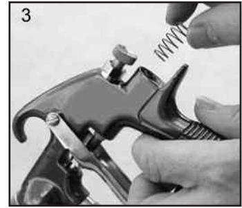
3. Remove Housing (10) and Air Valve Spring.
