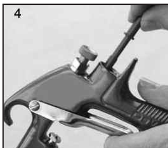
4. Retirer la soupape (11).
