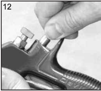
12. Fit Valve Seat to Gunbody.
