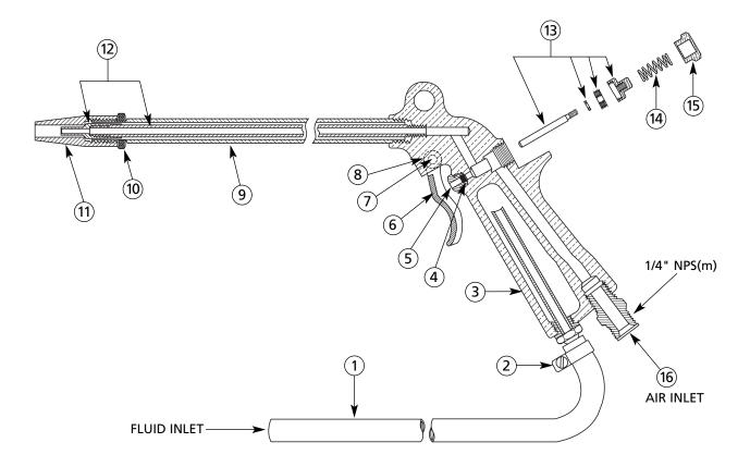
The Binks Model 140B spray gun is used for spraying solvents to clean engines and other machinery. Gun has a brass body with a ten inch nozzle/tube length. Flexible tubing is attached to the gun handle with a hose clamp for siphoning solvent from container. 1/4" NPS(m) air inlet. Requires 14 CFM air at 50 PSI. Working CFM can range from 8-1/2 to 18-1/2 CFM and from 40 to 100 PSI. Gun weight (less hose): 1.37 lbs.
