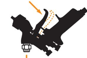
2. Use slight downward pressure. Use stem lugs for secure connection to lip on the adapter.
