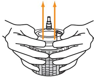
With the lid tab facing away, use forefingers to open lid. Allow paint to drain from the lid into the cup prior to opening completely.
