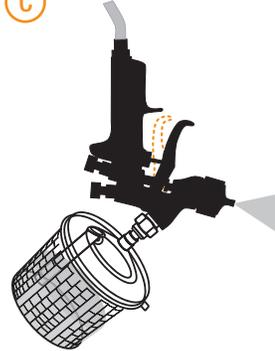
Connect hose, squeeze trigger, and purge air valve prior to painting.
