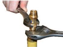
2.) Attach to tool or Desiccant Snake. Use TWO wrenches to tighten indicator. DO NOT over tighten. When using with Desiccant Snake the Indicator should be placed between the Snake and the spray gun.
