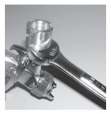
2. Tighten set screw firmly into gun hook.
