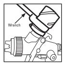
3. Using an 11/16" open end wrench, install the adapter by engaging the guick change tabs.
