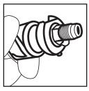
1. Place locking collar with set screw onto adapter.
