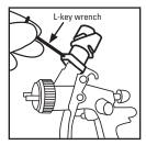
4. Tighten the set screw on the collar to prevent the adapter from disengaging.
