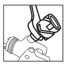
Using an 11/16 wrench, install the adapter (without the collar) tightly into the spray gun.
