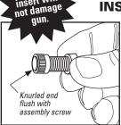
1. Install insert on screw until knurled groove end is flush.
