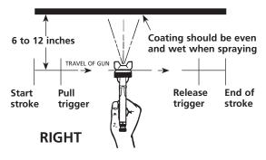
The distance between gun and surface should be 6 to 10 inches depending on material and atomizing pressure. The material deposited should always be even and wet. Lap each stroke over the preceding stroke to obtain a uniform finish.
