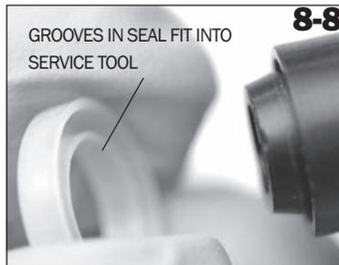
GROOVES IN SEAL FIT INTO
